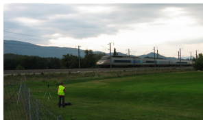
Acoustic measurement along a high speed track
